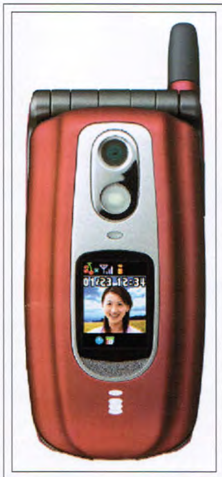
Fig. 1: The Fujitsu F505iGPS cellular phone uses a Pioneer full-color passive-matrix sub-display that incorporates UDC's red-emitting PHOLED material. The sub-display has a 1.1-in. diagonal, 96 \times 72 pixels, and 4096 colors.
